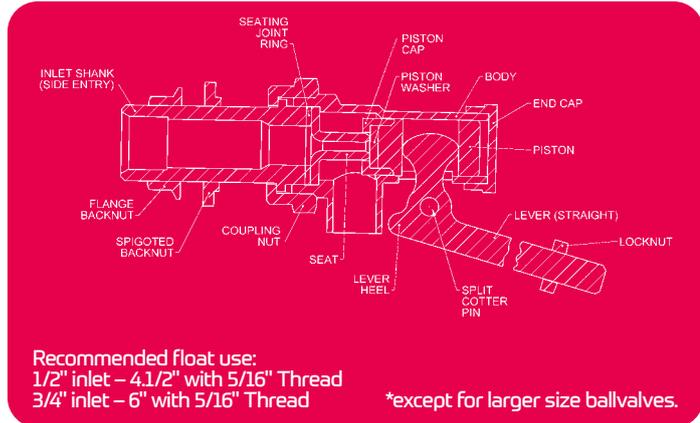
Our Brass Ballvalves forms part of our range of manual valves & tank fittings & are used widely in general services, water treatment & plumbing & heating applications, controlling the level of water into water tanks & cisterns.
